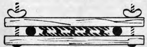
END VIEW OF SCREW BLOCK, SHOWING HOW CARDBOARD HOLDS SMALL CANES IN PLACE.
