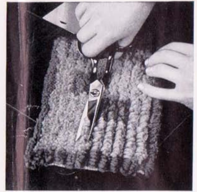
No. 8 Shearing Pile
